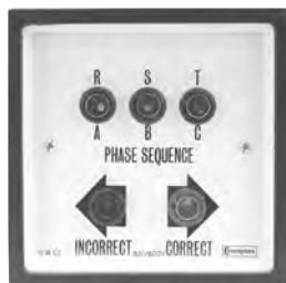
Electronic phase sequence indicators ensure correct phase rotation and the presence of all 3-phase supplies. Incorrect or loss of phase can cause serious damage in a wide range of electrical machines. Ship-to-shore supplies, mobile generators and remote installations are particularly vulnerable to this problem.
