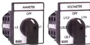
Panel mounted selector switches offer a 7-position voltmeter switch and a 4-position ammeter switch for reading line-to-line or line-to-neutral voltage and phase current.
