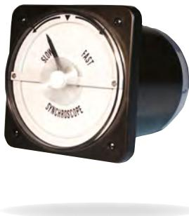
The Crompton Instruments AC synchroscope measures and displays the frequency difference of two power sources. Monitoring the display allows the user to connect two synchronized AC power systems together. This can help prevent the potential damage caused by connecting two unsynchronized power sources.
