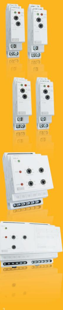
AC current protectors provide a continuous surveillance of monitored circuits and offer user adjustable trip points (set points) with time delay settings. When the current moves outside the set point limit for longer than the time delay, the relay will operate providing an alarm control or tripping signal.
