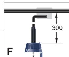
Insulated flexible line lead to fit to piercing connectors
