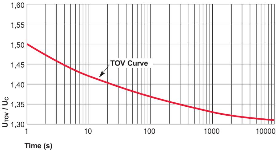
Samples are pre-heated to a temperature of 60° C according to IEC 60099-4, Ed 2,0 2004. Samples were subjected to a pre-stress equivalent to one high current impulse of 100kA, 4/10  $\mu$ s as per switching surge operating duty test.
