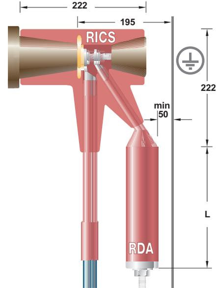
Gas insulated switchgear with RDA arrester and RICS adapter.
