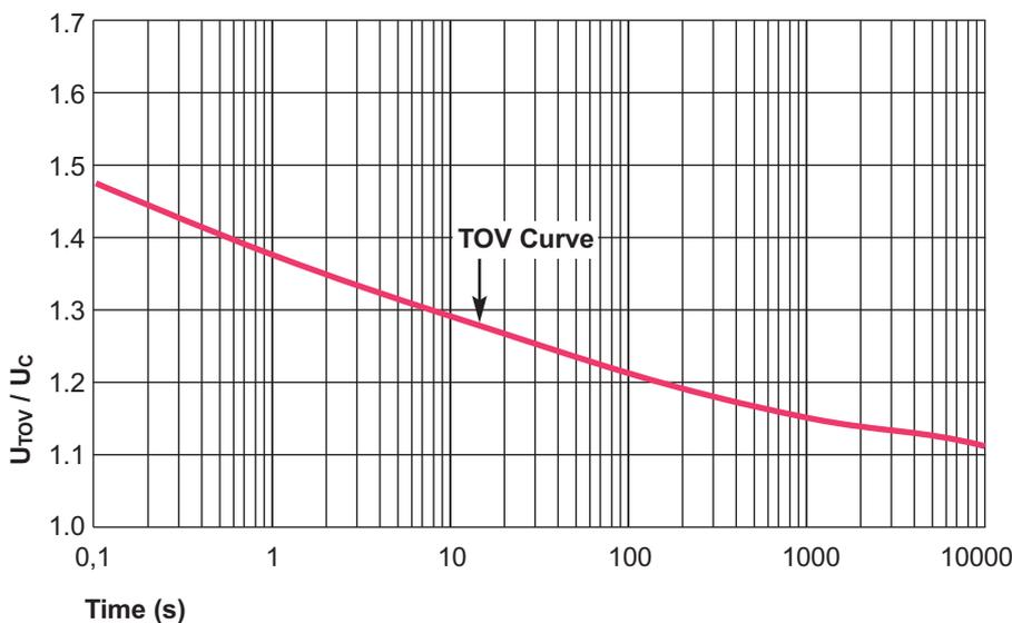
Samples are pre-heated to a temperature of 60° C according to IEC 60099-4, Ed 2,0 2006. Sample was subjected to a pre-stress equivalent to one high current impulse of 100kA, 4/10  $\mu$ s as per switching surge operating duty test.
