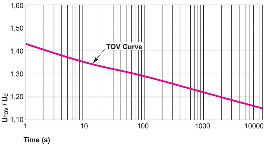
Samples are pre-heated to a temperature of 60° C according to IEC 60099-4, Ed 2,0 2004. Sample was subjected to a pre-stress equivalent to one high current impulse of 100kA, 4/10 μs as per switching surge operating duty test.
