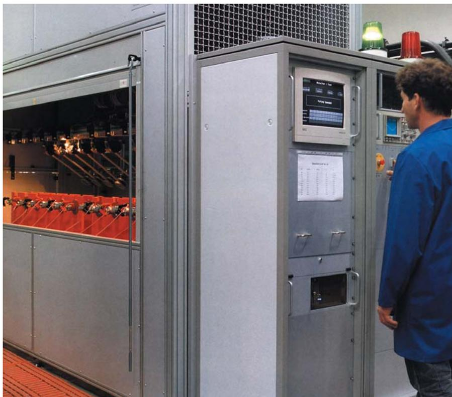
Automized routine test facility for Metal-Oxide Surge Arresters in the manufacturing area
