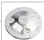
M5 Pedestal base with 4 holes on 280mm PCD or 3 x 15mm slots on 200mm - 254mm PCD
